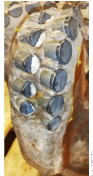
Two views showing GTD55DKOs dull condition of 1-1-CT-S-X-I-WT-TD after a long, hazardous run.
